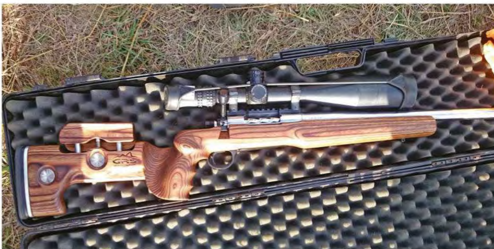
A 6x47mm built on a MOJET action for competitive sport shooting but with the correct twist barrel and suitable high BC bullets, is quite capable of connecting on steel out to 1 250m.
