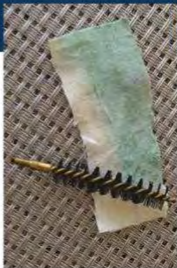
LEFT: A properly free-floated barrel with a business card in the gap between the barrel and the stock. CENTRE: After removing nitro fouling, you need to remove copper fouling – manifested here as a green deposit on the cleaning patch. RIGHT: Pushed through from the chamber end, this cleaning patch shows copper particles from my .375H&H barrel after firing Barnes-X bullets.
