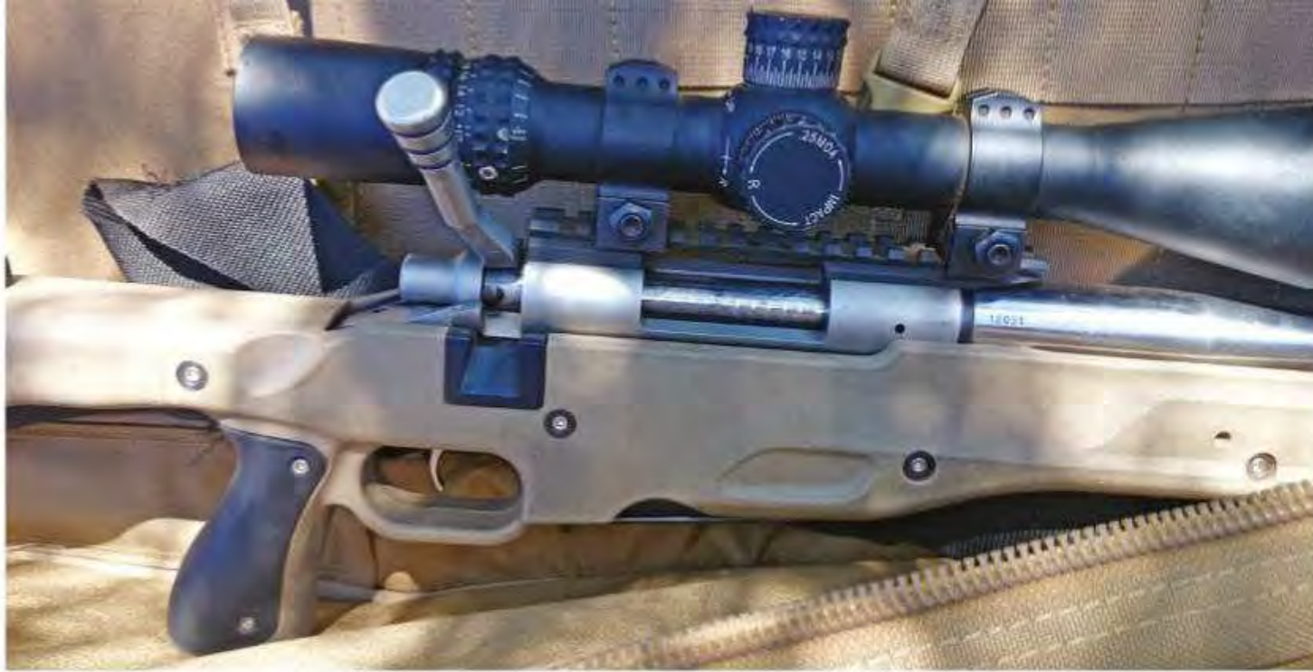
Modified Rem 700 Short Action in stainless steel used for building a 6.5mm Creedmoor.
