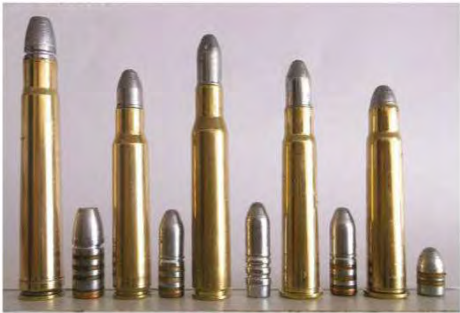
L-R: Cast bullet loads and the bullet used: .375 with 246gr gas-checked bullet from Lyman mould; 8mm Mauser with 175gr bullet from Lee mould; .30-06 200gr bullet from Lee mould; .303 with 185gr bullet from Lee mould; .303 with 88gr bullet from RCBS mould.
