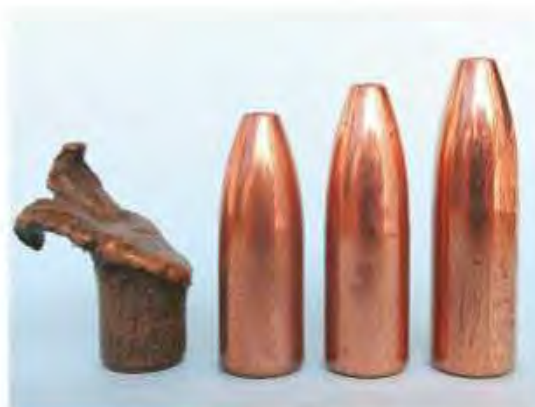
LEFT: Four Barnes-X .458 bullets. L-R: (1) Recovered 400gr that penetrated the cow's head and three or four neck vertebrae; (2) Same 400gr unused; (3) 450gr preferred by author for its higher SD; (4) 500gr: its length requires compressed loads in a .458 Lott.
